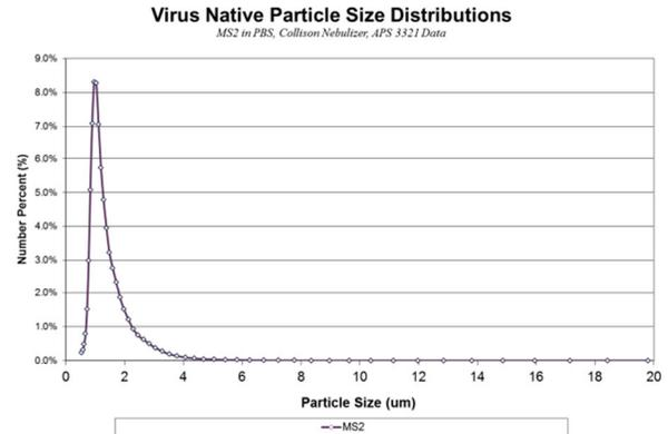
**Figure 4:** Viral Particle Size Distribution in Test Chamber.
