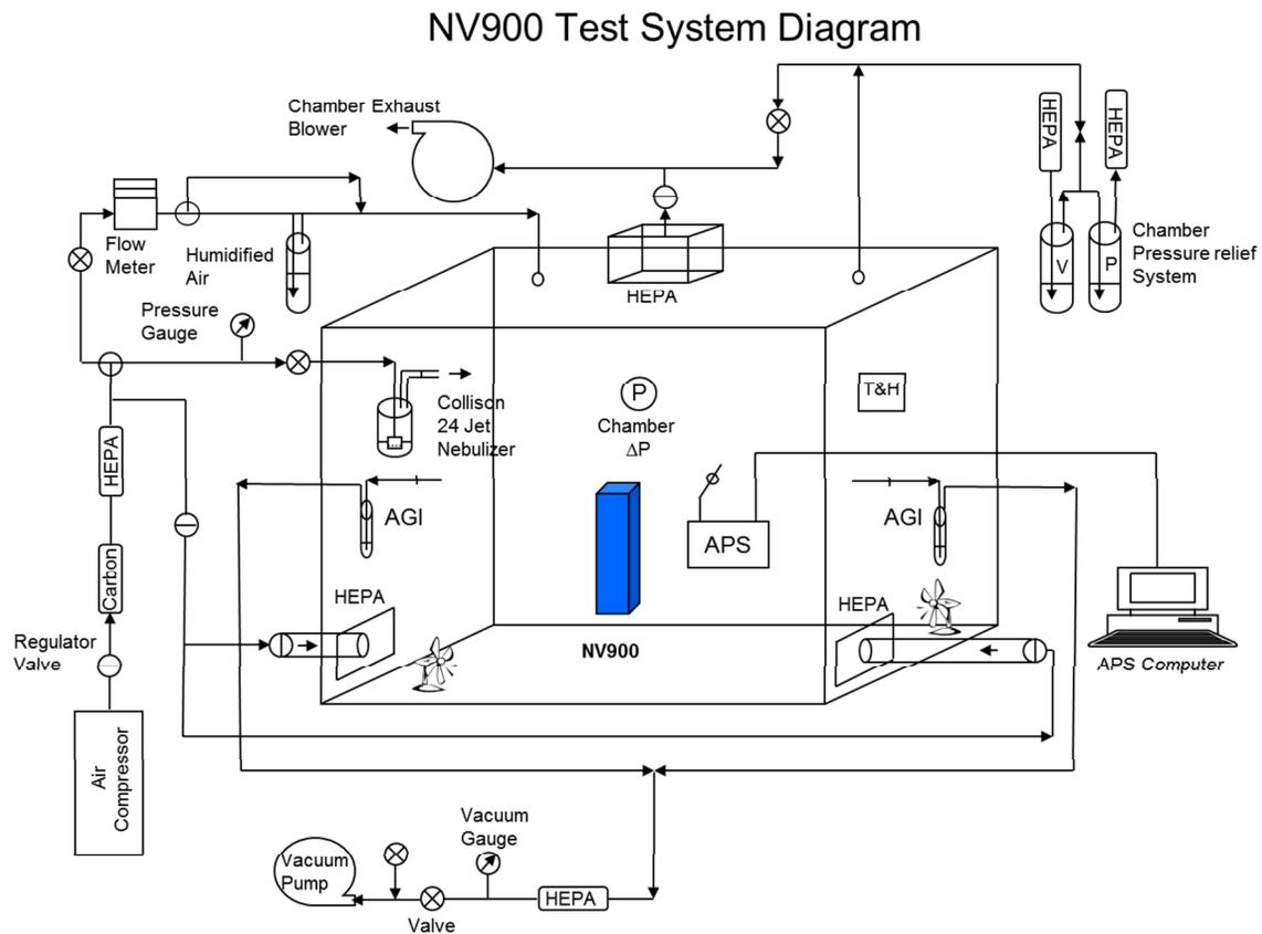
Figure 2: Bio-Aerosol Test Chamber Flow Diagram.
