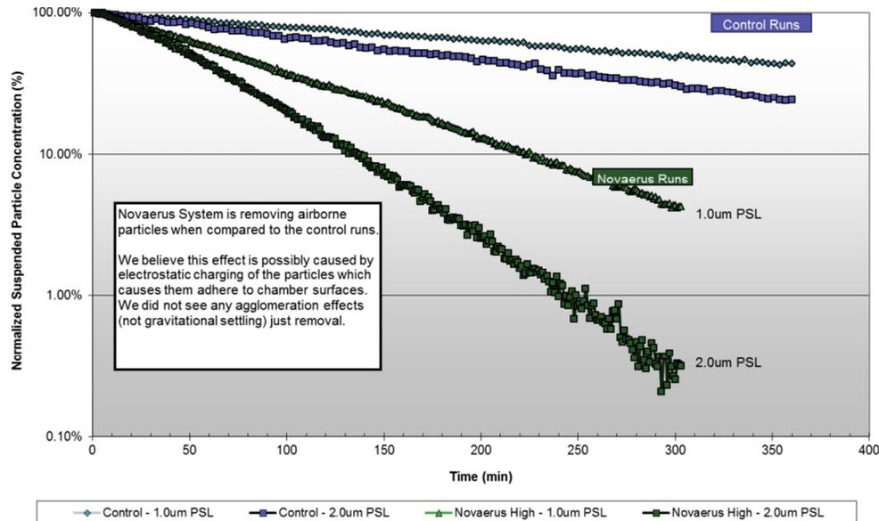
Figure 3: Preliminary PSL Trials Chamber and NV900 Characterization.
